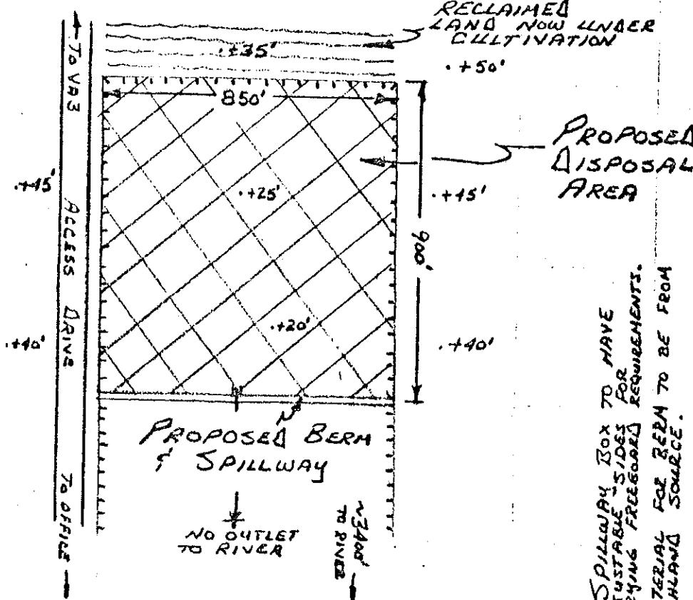
NOTE: SPILLWAY BOX TO HAVE ADJUSTABLE SIDES FOR VARYING FREEBOARD REQUIREMENTS. MATERIAL FOR BERM TO BE SOIL AND HAYLAND SOURCE.
